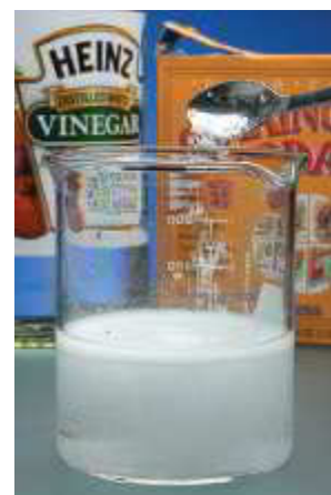
When sodium bicarbonate (baking soda) reacts with an acid (vinegar), the products are carbon dioxide gas, water, and a salt.
