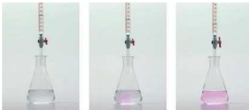
FIGURE 10.6 The titration of an acid. A known volume of an acid is placed in a flask with an indicator and titrated with a measured volume of a base solution, such as \text{NaOH} , to the neutralization endpoint.
