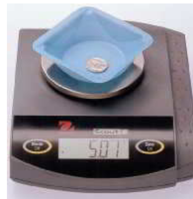
FIGURE 2.3 On an electronic balance, the digital readout gives the mass of a nickel, which is 5.01 g.
