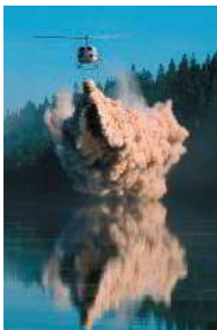
A helicopter drops calcium carbonate on an acidic lake to increase its pH.
