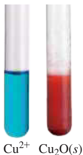
FIGURE 12.8 The blue \text{Cu}^{2+} in Benedict's solution forms a brick-red solid of \text{Cu}_2\text{O} in a positive test for many sugars and aldehydes.
