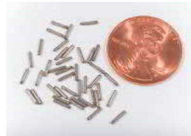
Titanium “seeds” filled with a radioactive isotope are implanted in the body to treat cancer.
