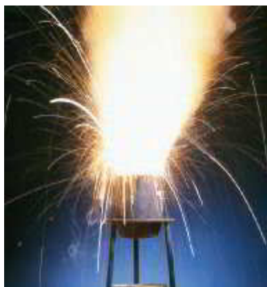
The high temperature of the thermite reaction has been used to cut or weld railroad tracks.
