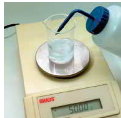
Add water until the solution has a mass of 50.00 g When water is added to 8.00 g of KCl to form 50.00 g of a KCl solution, the mass percent concentration is 16.0% (m/m).
